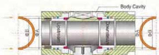
When the medium in the upstream or downstream of the valve, since  $\Phi A > \Phi B$ , the pressure differential makes the medium push the seats to the ball, to achieve a reliable seal.
